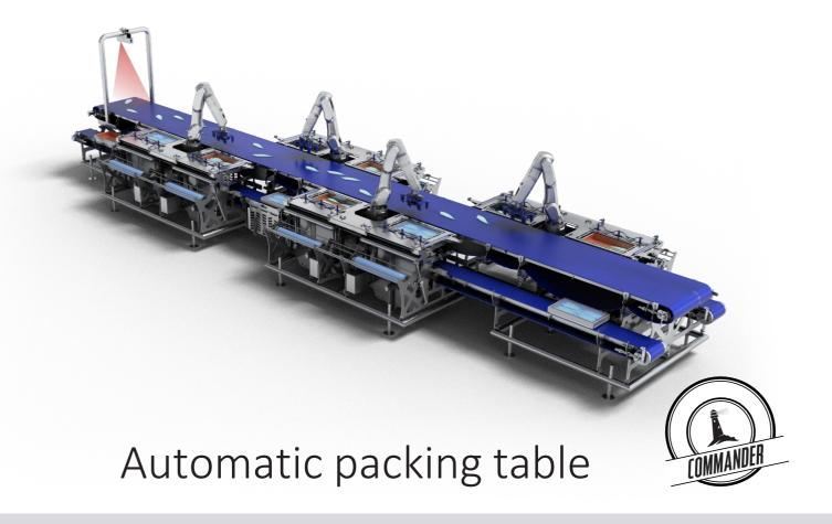
By using advanced automation and robotics, the automated packing table offers interleaving packing solutions for fish filet.
